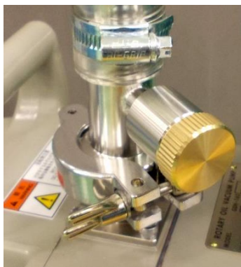
Pump Leak Valve
